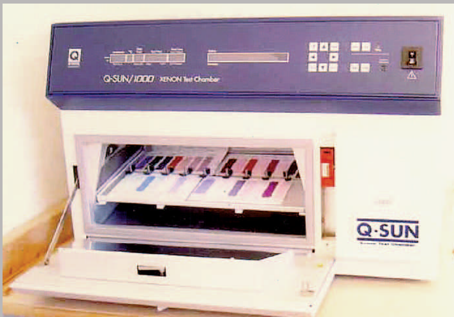
A table top xenon tester with the door open and pastel samples inside
