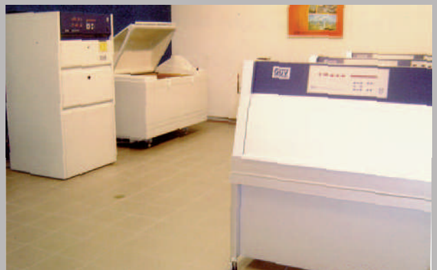
A variety of testing instruments used by Gottsegen: from left, a lab-sized xenon tester, a salt-spray chamber, and a fluorescent light instrument
